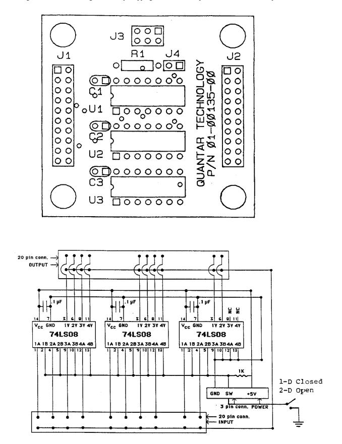
Figure 3-18A MCA Interface, Mounted On Main Board, Schematic and Component Locator, for S/N 7440 and above
