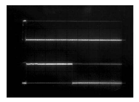
Figure 3-8 Upper trace, STROBE (10 bit, negative polarity); Lower, XY Position; Vert=2 V/cm, Horiz=2 µsec/cm
