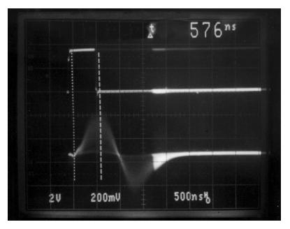
Figure 3-6 Upper, RATE pulse; Lower, SUM pulse: Vert=2 V/cm, Horiz=500 nS/cm
