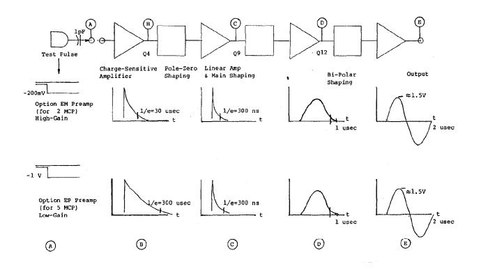
Figure 3-3 Charge Amplifier/Shaper Block Diagram and Timing
